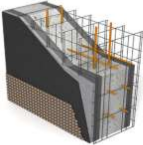
FOUNDATIONS & CELLARS Lattice + infill material + tanking
